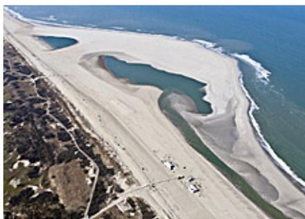
The Sand Engine will fortify eroding beaches as ocean currents slowly redistribute its dredged material.
