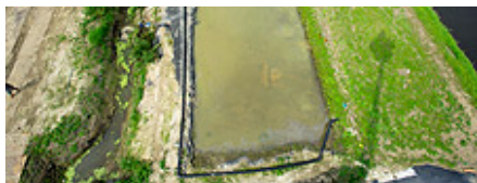
A “Smart Dike,” which contains sensors that relay real-time status reports on the condition of the dike to decision makers. DELTARES
