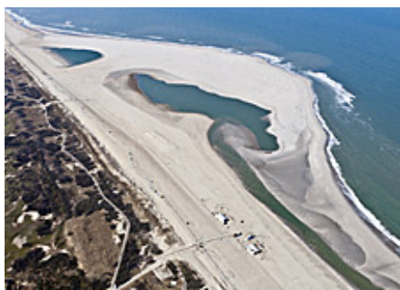
The Sand Engine will fortify eroding beaches as ocean currents slowly redistribute its dredged material. RIJKSWATERSTAAT/JOOP VAN HOUTD
